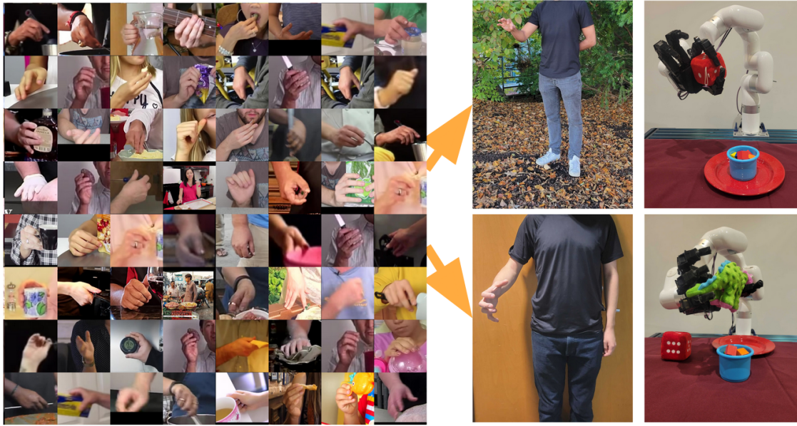
Figure 3.1: Our system leverages passive data from the internet to enable robotic real-time imitation in-the-wild. This low-cost system does not require any special gloves, mocap markers or even camera calibration and works from a single RGB camera.
