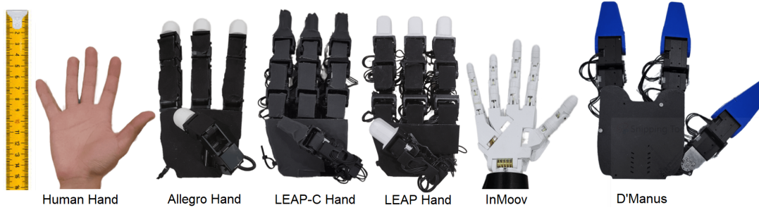
Figure 2.1: Relative size of popular robot hands to scale. Left to right , adult human hand, Allegro Hand [6], LEAP-C Hand, LEAP Hand, Inmoov [21], D’Manus [70]. LEAP Hand is similar in size to Allegro and \sim 30\% larger than a human hand. D’Manus is considerably larger than the rest. Because of the tendon-driven nature, Inmoov is the smallest robotic hand. The hands are accurate to scale.
