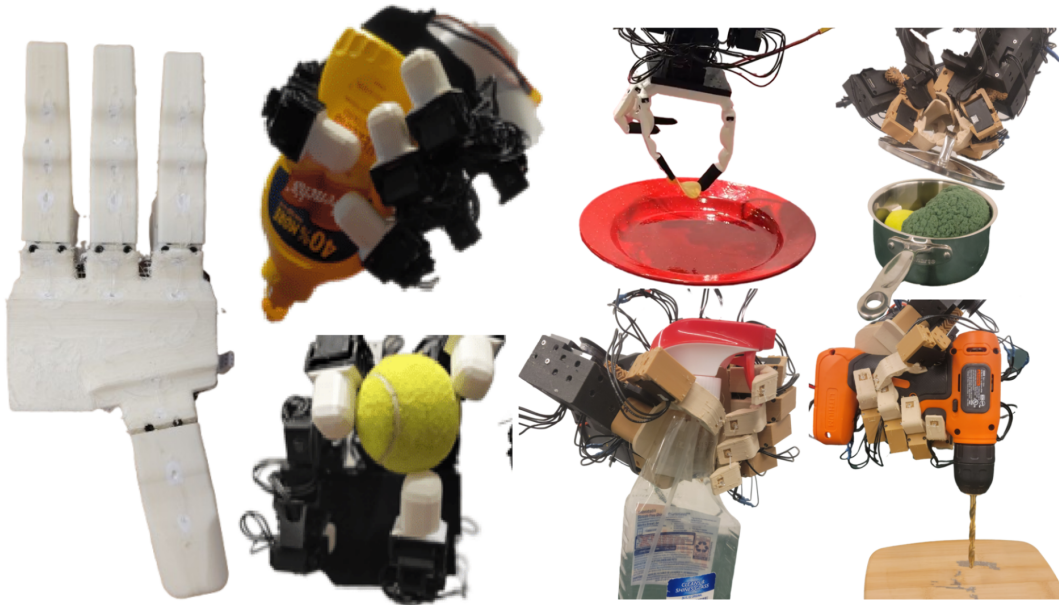
Figure 8.1: Our demonstration will feature four different low-cost, open-source robotic hand designs, including a new model introduced in this paper, LEAP Hand V2. (left) These hands are highly dexterous, easy to build, durable, and affordable. We also provide a suite of open-source software tools, including motion capture teleoperation, human video-based learning, and reinforcement learning capabilities. Building on our successful demonstrations at RSS 2023 and 2024, we aim to further highlight the potential of low-cost, open-source robotic hands and strengthen our open-source robot hand community at RSS 2025. Please visit our website at https://leaphand.com for more details. for this demonstration—alongside our previous robot hands with real robot interactive demos. Following our successful demos at RSS 2023 and 2024, we will again offer an engaging opportunity for attendees to get hands-on experience and information about the accessibility of low-cost, open-source robotic hands. Please visit our website at https://leaphand.com
