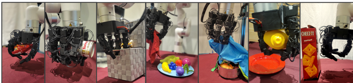
Figure 4.5: Tasks used in experiments. From left to right: pick, rotate, open, cover, uncover, place and push. See https://video-dex.github.io for videos of these tasks.
