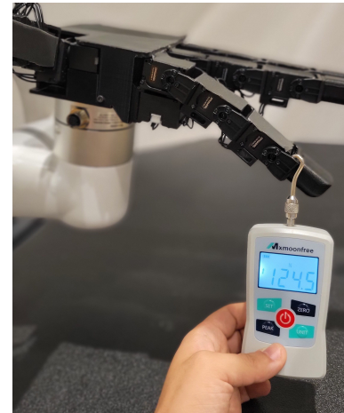
Figure 2.7: Pullout Test. A pull-out force is applied and the maximum force is recorded before the hand has a 15 error or slipping.
