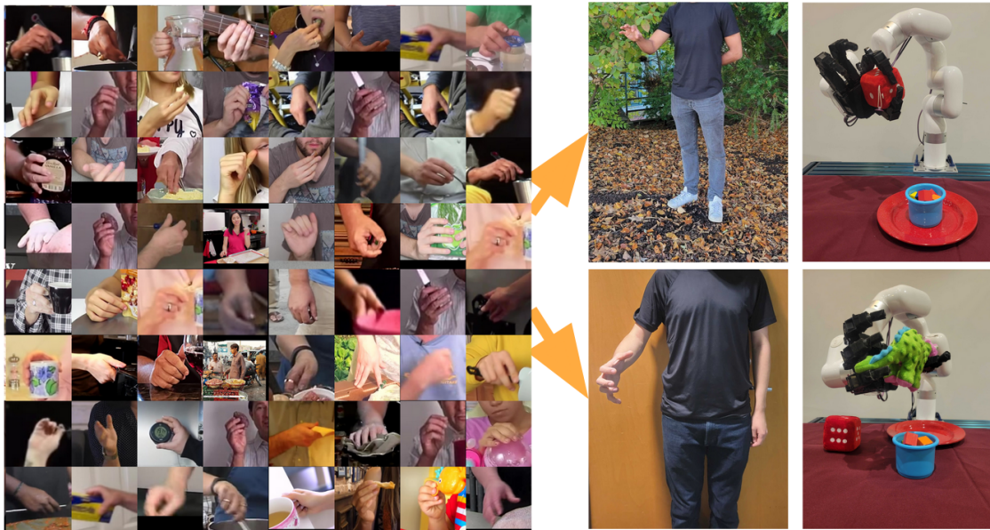
Figure 3.1: Our system leverages passive data from the internet to enable robotic real-time imitation in-the-wild. This low-cost system does not require any special gloves, mocap markers or even camera calibration and works from a single RGB camera.
