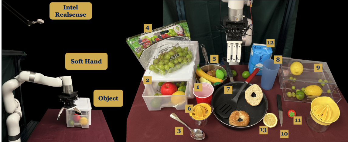
Figure 6.4: Left: Workspace Setup. We place an Intel RealSense camera above the robot to maintain an egocentric viewpoint, consistent with the affordance model’s training data. Right: Thirteen objects used in our experiments.
