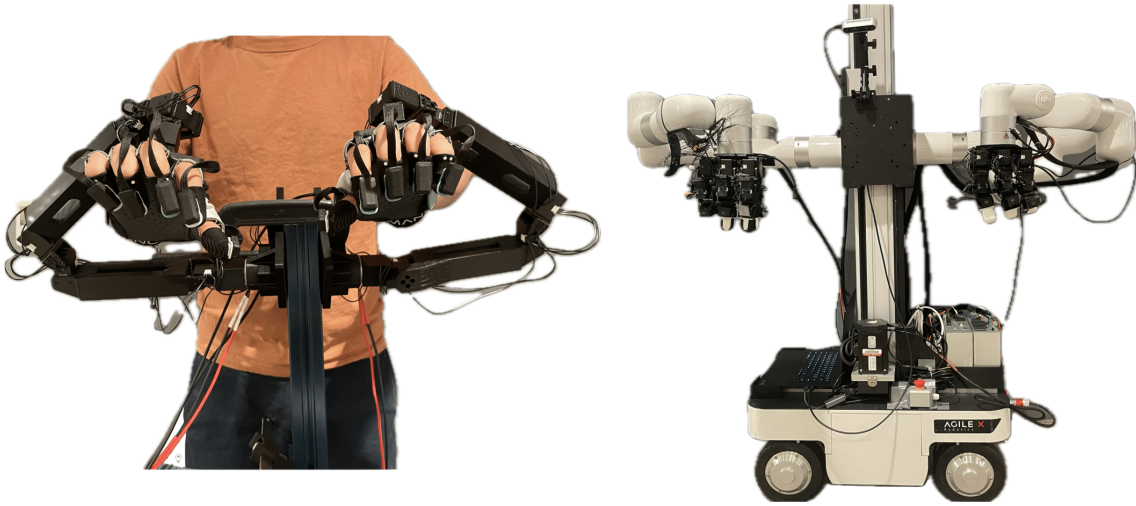
Figure 9.2: Mobile bimanual teleoperation system Left: An operator strapped into BiDex. Right: Our bimanual robot setup including two xArm robot arms, two LEAP Hands [339] and three cameras on an AgileX base.
