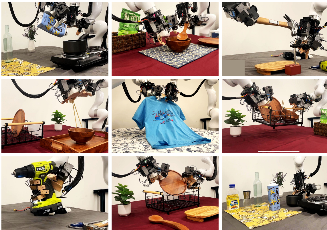
Figure 9.1: Bimanual Dexterity: BiDex can effortlessly teleoperate various complex tasks including pouring, scooping, hammering, chopstick picking, hanger picking, picking up basket, drilling, plate pickup and pot picking to train high-quality behavior cloning policies with over 50 degrees of freedom. Our teleoperation system and two LEAP hands [339] costs around $12k in total and is readily reproducible by academic labs.
