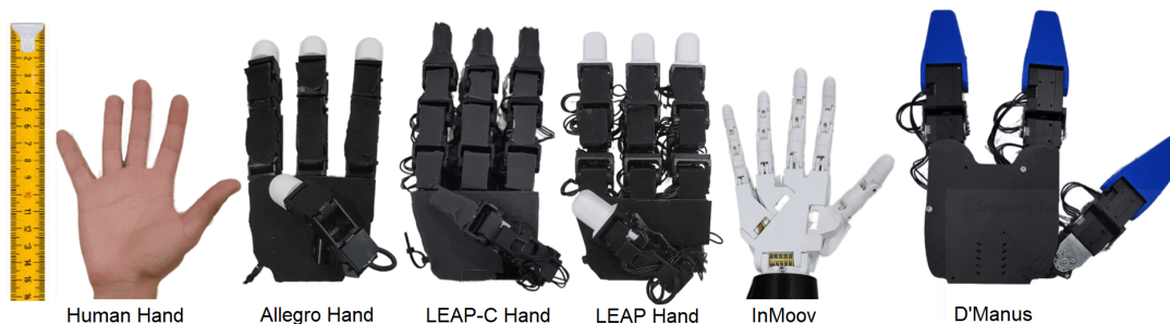
Figure 2.1: Relative size of popular robot hands to scale. Left to right , adult human hand, Allegro Hand [7], LEAP-C Hand, LEAP Hand, Inmoov [22], D’Manus [75]. LEAP Hand is similar in size to Allegro and \sim 30\% larger than a human hand. D’Manus is considerably larger than the rest. Because of the tendon-driven nature, Inmoov is the smallest robotic hand. The hands are accurate to scale.
