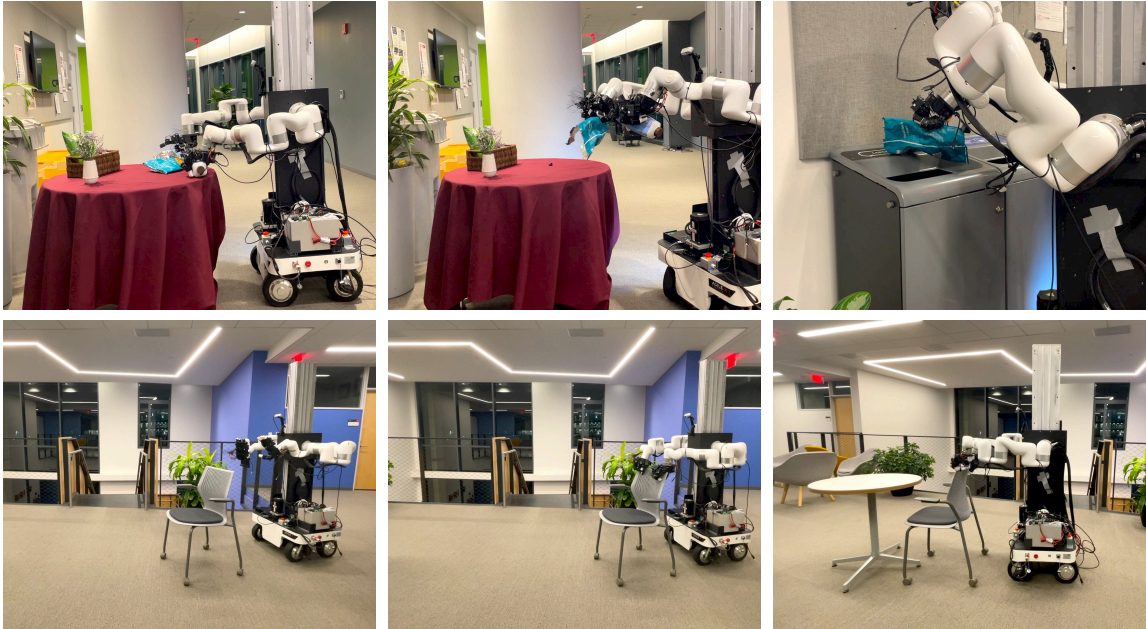
Figure 9.3: All Tasks: Teleoperation of the mobile robot systems with BiDex. Top: Picking up trash from a table and discarding it into a bin. Bottom: Grasping a chair and moving it to align with a table.
