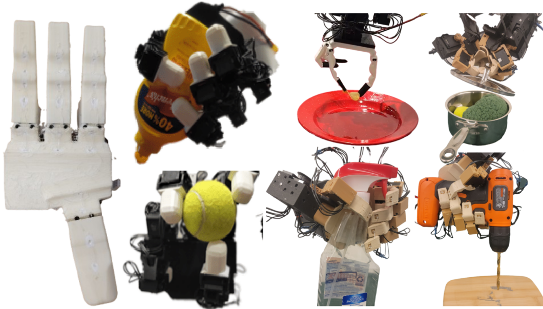
Figure 8.1: Our demonstration will feature four different low-cost, open-source robotic hand designs, including a new model introduced in this paper, LEAP Hand V2. (left) These hands are highly dexterous, easy to build, durable, and affordable. We also provide a suite of open-source software tools, including motion capture teleoperation, human video-based learning, and reinforcement learning capabilities. Building on our successful demonstrations at RSS 2023 and 2024, we aim to further highlight the potential of low-cost, open-source robotic hands and strengthen our open-source robot hand community at RSS 2025. Please visit our website at https://leaphand.com for more details.
